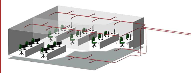
Having a backup system is advisable to ensure protection during charging and/or re-stamping of the main system, and when the system covers several areas via selector valves.
